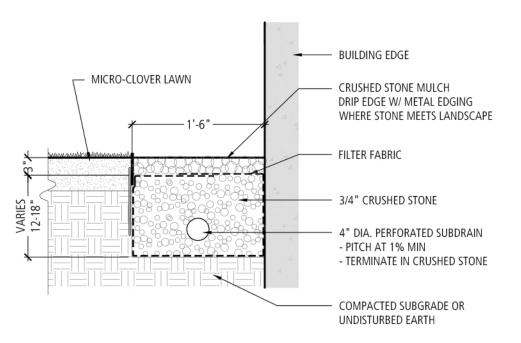
Detail: Proposed Crushed Stone Drip Edge w/ Perforated Subdrain
